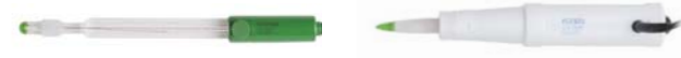
HI10480 PTFE reference, double junction, Clogging Prevention System (CPS), glass body pH electrode with temperature sensor Recommended for wine analysis and solutions with a high concentration of suspended solids FC2320 Open viscolene reference electrolyte, double junction, PVDF body pH electrode with conical tip and temperature sensor Recommended for meat applications with use of optional FC098 20 mm (0.8") or FC099 35 mm (1.4") stainless steel blade
